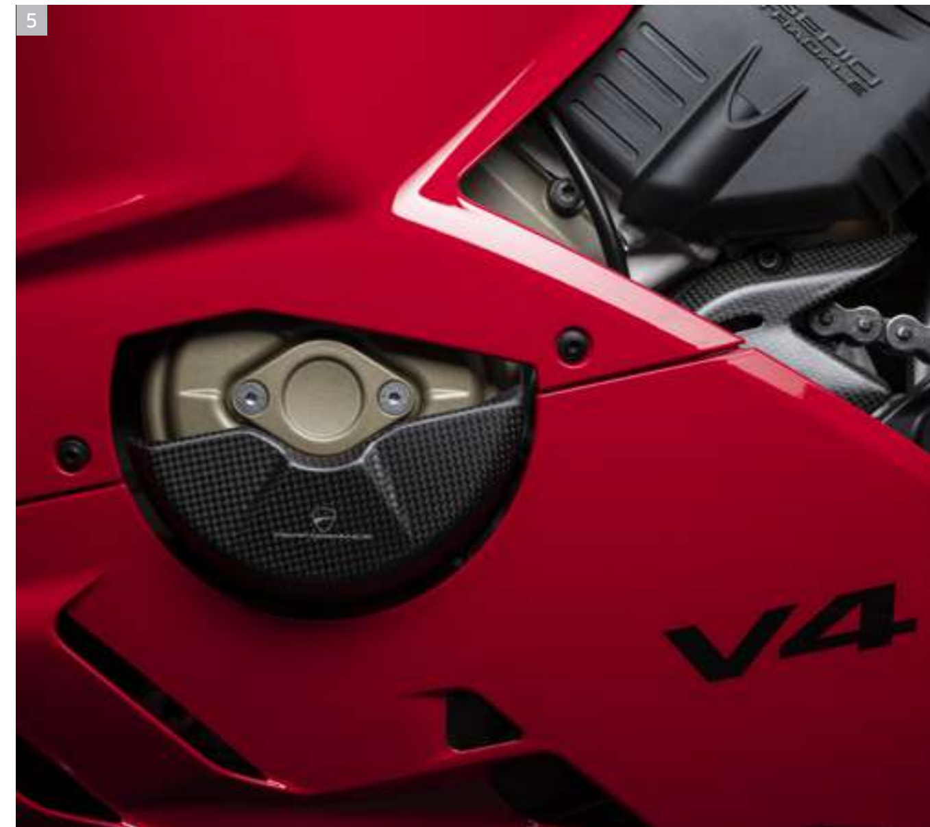
5 Carbon protection for generator cover.
