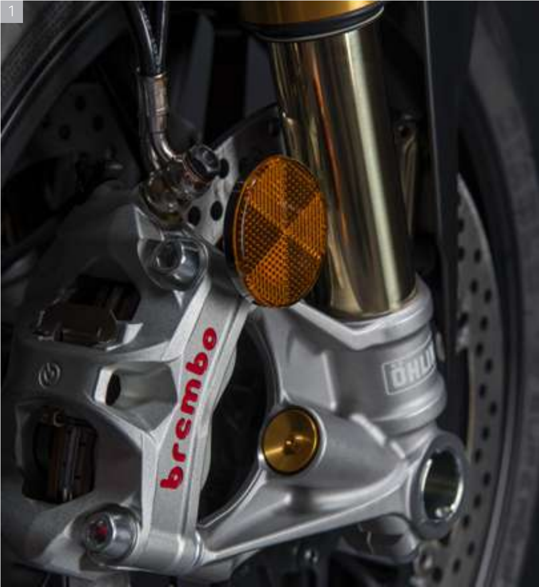
1 Öhlins 43 mm NPX25/30 pressurised fork
